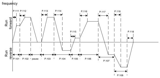
• The run direction is set in binary form (8-bit), and then translated to decimal form and stored in P.121. "1" means run forward, and "0" means run reversely. The highest bit is the run direction of section 8, while the lowest bit is the direction of the section 1.
