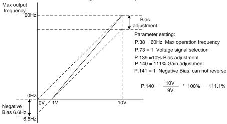
Example 7: This example integrates all the application of potentiometer. Together with the application of forward and reverse rotation, it fits in the system easily for assorted complicated application. Please be cautious that when setting up this application, the forward and reverse rotation commands of the external terminal will be disabled automatically.
