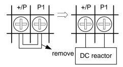
Note: Frame C, E and F corresponded inverters have built-in DC reactor.
