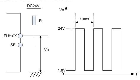
Note: 1. Fu and 10X share the same hardware terminal. When switching the function (change the value of P.74), the pin slot on the control panel needs to be switched at the same time. The initial position of the slot cover is at FU.
