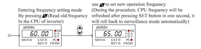
Press the MODE key to enter the frequency setting mode.
