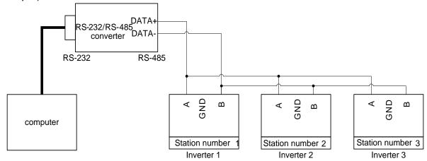
SF series inverters have two types of communication protocols: Shihlin communication protocol and MODBUS communication protocol.
