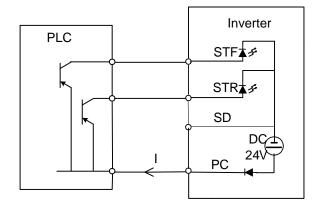
Source Input: the multi-function control terminal is connected directly with open-emitter PLC
