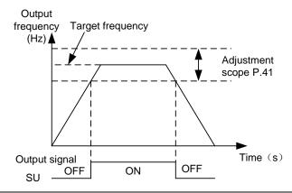
Note: In this paragraph, SU is the function name for "multi-function output terminal". Please refer to <u>P.40</u>, P.85, P.129 and P.130. For wiring, please refer to Section 3.5.
