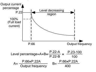
Note: When  $\underline{P.300}$ =3 for sensorless vector control is selected from  $\underline{P.300}$  control method, P.22 will be used for the torque limited horizontal operation.
