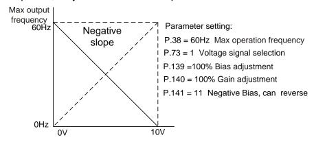
Note: 1. In "External mode", "combined mode 2" or "combined mode 4", the target frequency of the inverter will be determined by the signal between 2-5/4-5 terminal when RH, RM, RL and REX are all "off."
