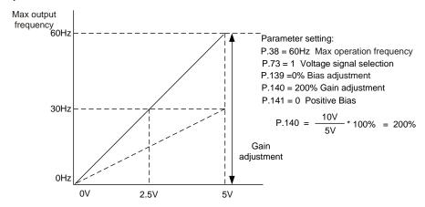
Example 5: This example is a typical negative bias application. An advantage of using negative bias is its anti-noise interference effect. Under an unfavorable application environment, it is recommended to avoid using a signal that is less than 1V to set up the operation frequency of the AC motor drive.
