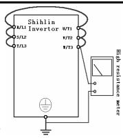
Note: Please do not carry out a high-voltage test; as such test will damage the built-in semiconductor components.
