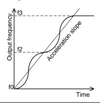
Note: this pattern can effectively reduce motor vibration during the acceleration / deceleration, and thus prevent the belts and gears from broken.
