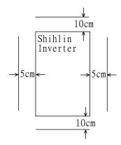
3. The ambient temperature shall not exceed 4. Install the inverter at a correct position in a the permissible value.
