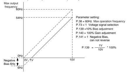
Example 6: This example is an extension of Example 5. The maximum operation frequency can be obtained by including the gain calibration. The wide application of this example offers the users good flexibility.
