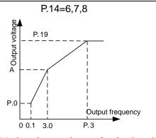
When P.14=6, the value of A is 8.7%. When P.14=7, the value of A is 10.4%. When P.14=8, the value of A is 12.0%.(Note 2)
