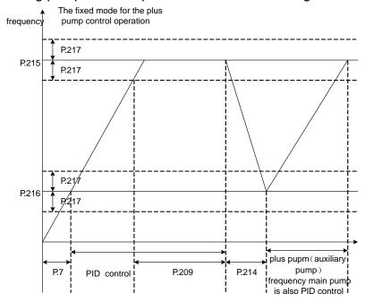
When the inverter is running, if the pressures command (or the frequency command) is larger than the feedback value continuously, PID output (equals to the output frequency) will increase until reaching the maximum frequency (P.215). This state will continue until the time assigned by P.209. If the bias between the command value and the feedback value is larger than the set value of P.217, increasing pump control will be performed.
