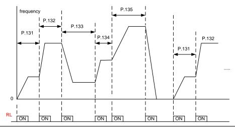
Note: 1. The inverter can run eight levels of speed in the procedure, and the frequency is determined by P.131~P.138.
