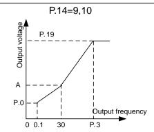
When P.14=9, the value of A is 20.0%. When P.14=10, the value of A is 25.0%.(Note 2)
