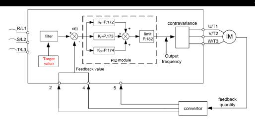
When the output frequency reaches the set value of P.182, the feedback value will be less than the product of the target value and P.172. In addition, when the duration lasts more than the set value of P.176, PID will be considered as abnormal and handled according to the set value of P.177.
