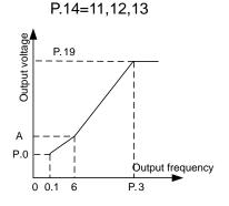
When P.14 = 11, the value of A is 9.3%. When P.14 = 12, the value of A is 12.7%. When P.14 = 13, the value of A is 16.1%. (Note 2)
