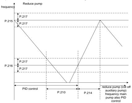
When the inverter is running, if the pressure command (or the frequency command) is smaller than the feedback value continuously, PID output will decrease until reaching the minimum frequency (P.216). This state will continue until the time assigned by P.210. If the bias between the command value and the feedback value is larger than the set value of P.217, decreasing pump control will be performed.
