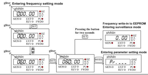
Note: 1. Use or to change the frequency when the inverter is running.
