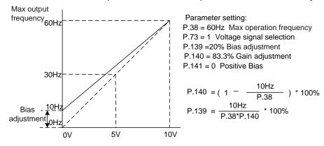
Example 4: This example uses 0~5V to set the frequency. Besides adjusting the method of gain, the user can also set P.38 to 120Hz or P.73 to zero to attain the same operation.
