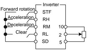
Wiring of the remote control setting
