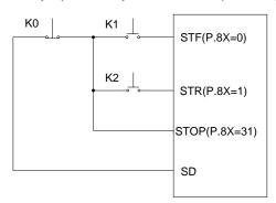
(4). Three-wire control mode 2 (with self-maintenance function): K1 is for the STOP function that is normally close. When it is open, the inverter will stop. K2 is the RUN signal that is normally open. It indicates that pulse signal is active, i.e., jog is valid. For the direction changing signal (STF/STR), the parameter corresponds to the external terminals is 39. When changing the direction, stop the inverter first, RUN the inverter before activating it.
