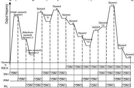
• Provided that the parameter set values of P.24~P.27 and P.142~P.149 are all 99999, the target frequency will be determined by RL, RM and RH these three speeds. See the table below (the priority of the terminals is RL>RM>RH):
