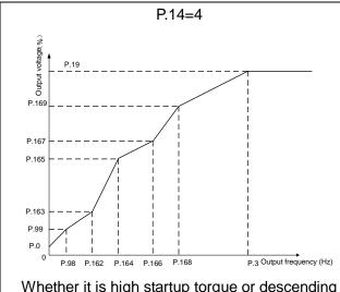
Whether it is high startup torque or descending torque, they are due to the set values (Note 1).
