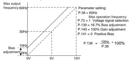
Example 3: This example is also frequently used by the industry. The comprehensive usage for all domain of the potentiometer setup elevates the flexibility.
