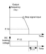
Note: To achieve the optimum control characteristics, P.11 and P.12 should be set properly.
