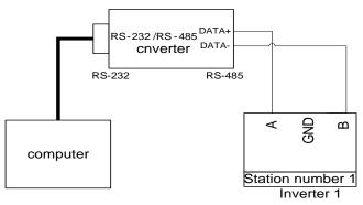
• Communication between the position machine and multiple inverters (take computer as an example).
