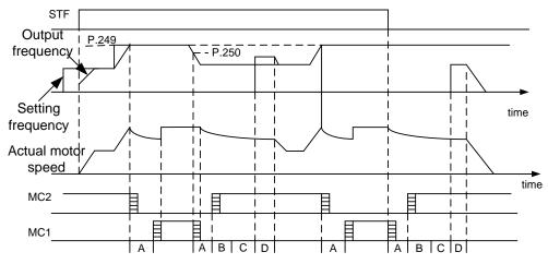
During the automatic switchover, A: P.247 MC switchover interlocking time; B: P.248 starting waiting time; C: P.57 restarting free operation time; D: P.58 restarting elevating time.
